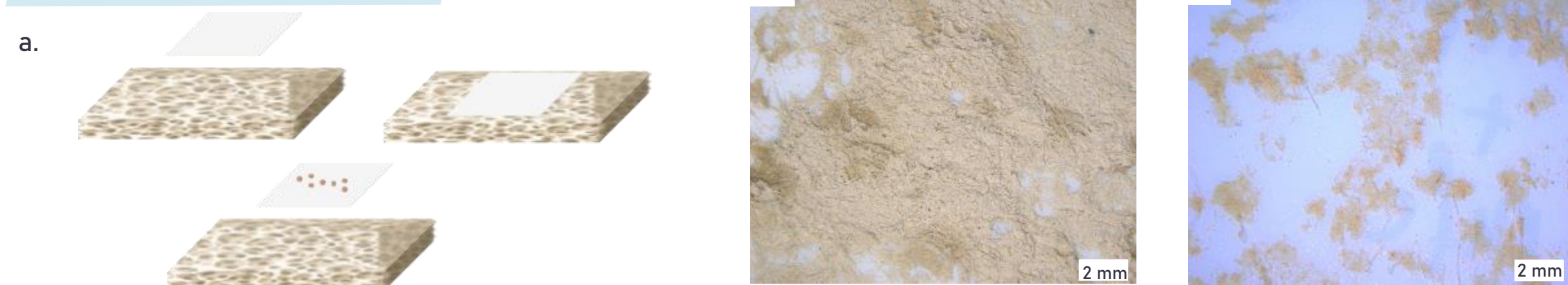
Figure 5: a. abrasion test setup, standard tape surface after abrasion; b. ONP ratio=1; c. ONP ratio=1 + 5% MFC in bulk; d. Percentage of foam's surface covered by dust.
