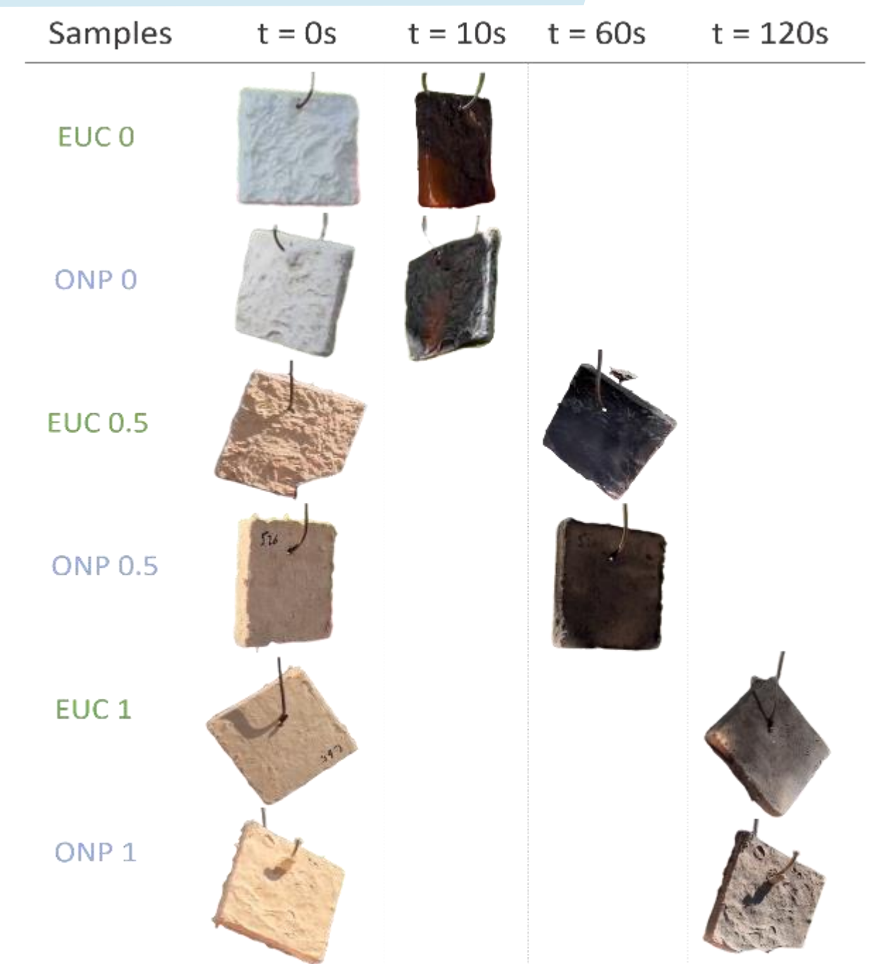
Figure 3: Fire resistance test on foam samples with eucalyptus or old newspaper pulp, with various earth/fibre ratios and their burning stages at 0, 10, 60 and 120 seconds.
