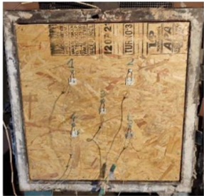
Sample 1, Side non exposed to fire
