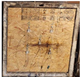
Sample 1, Side non exposed to fire. Test finished
