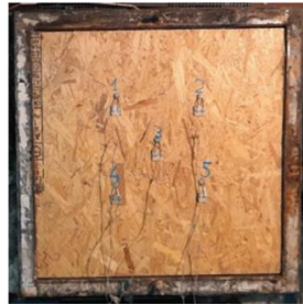
Sample 2, Side non exposed to fire
