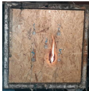
Sample 2, Side non exposed to fire. Test finished
