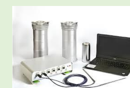
Calorimetry : Langavant Calorimeter following the NF EN 196-9.
