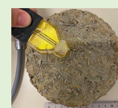
Thermal conductivity : Hot Disk with the 5501-probe model.
