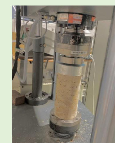
Compressive strength : On 3 cylindrical specimens (11x22 cm) using a hydraulic press with a loading speed of 5 mm/min
